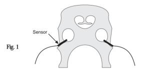
If pickup is too loose, shim with included shim material (see Fig. 2). If pickup is too tight, file the bridge slot slightly.
