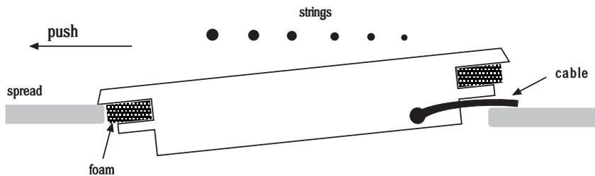
3. Lower the treble side of the pickup into the sound hole and release the pickup to center it.
