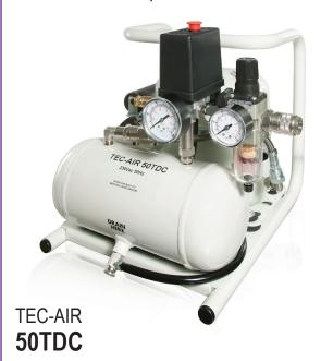
The tec-AIR 50TDC is an almost silent, compact air compressor. It weighs just 21 kilos (46lbs), and comes complete with a robust tubular carrying frame. It is rated at 50 l/min (2.15cfm) and works to a maximum pressure of 8 bar (120psi). It is capable of operating up to two pneumatic tec bead applicators or one pneumatic tec spray applicator intermittently for small area coverage. It can also be used with most other pneumatic tools such as staplers, air brushes and tyre inflators.
