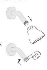
3. Slightly loosen the wing nut on the female connector side, pull the connector away from the wing nut and rotate it 180 degrees so it point outwards.
