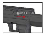
Rotate the Bolt Handle 90 degrees and remove from the body of the Rifle. Insert the Bolt Handle in the desired side of the Rifle and screw in the Retaining Bolt hand tight.
