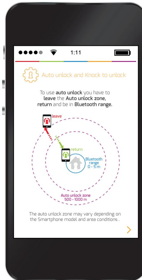
Prior to enable the auto unlock feature an explanation page will run through how the automatic unlock feature works. The GEO location determines your position when you enter the auto unlock zone approx. 500 - 1000 meters (1640 - 3281 feet) from your Danalock and unlocks your door when you get in Bluetooth range 0 - 5 meters (0 - 16.4 feet) from your door.
