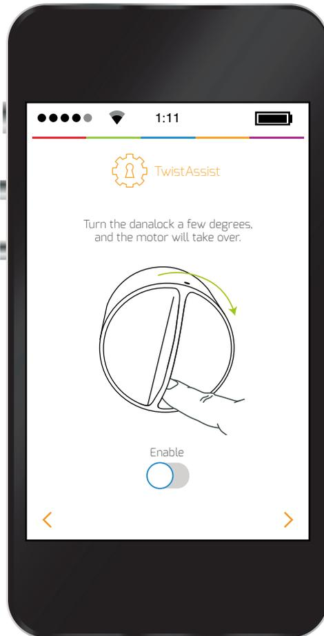
Enable Twist-Assist if you would like to unlock by turning the Danalock a few degrees making the motor take over.
