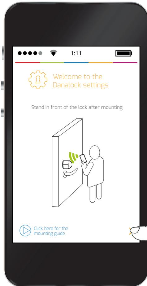
The Bluetooth signal has a range of 0 - 5 meters, so stand in front of your Danalock when you want to connect the Smartphone with it.
