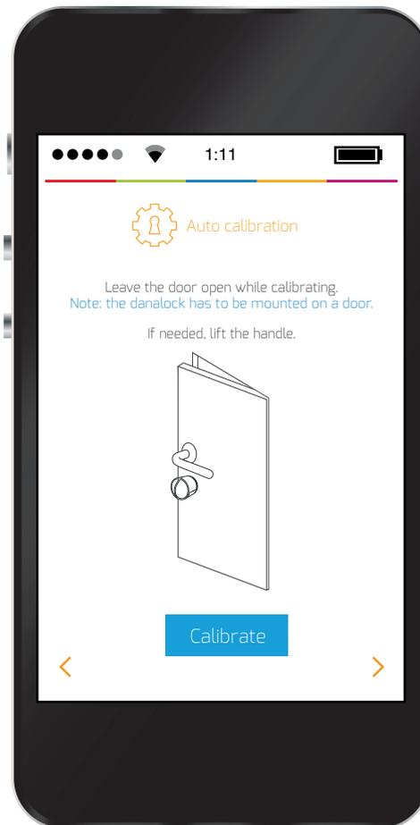
Now you calibrate your Danalock. Turn the Danalock manually until the door is unlocked and leave the door open while calibrating. Lift the handle if needed. Press the blue arrow at the right bottom corner to engage the calibration.
