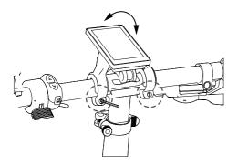
**Step 5.** Release the clamp under the handlebar, pull the handlebar up or push it down to adjust height to your desired, then close the clamp to secure handlebar in place.
