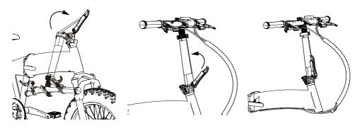
**Step 3.** Stand in front of the bike and clamp front wheel with both legs, verify the handle bars are straight and in line with the front wheel. Make sure the pinch bolts are tight and your cannot turn the stem freely from the front wheel. Sit on the saddle, adjust the handlebar to comfortable angle, and close the handlebar
