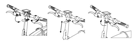
**Step 6.** Open the clamp under the seat post,set it to a height which fits the rider then close the clamp to secure the seat in place.
