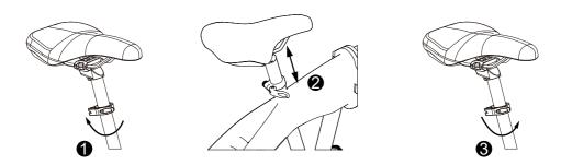
**Note:** Position the seat at the right height is key for better pedaling, safety and overall comfort. The rider's leg length is used to determine the seat's position. When pedaling, your hips should remain level and your legs should not over-extend. To determine the right seat height, sit on the eBike with pedal at its lowest point and place the ball of your foot on the pedal. If your knee is bent slightly at this position (about 60 degrees), the seat is at the right height.
