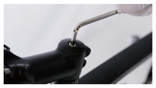
5.Align the stem so the handlebar is perpendicular to the front wheel. Use the allen wrench to tighten the stem clamp bolts evenly (a half turn at a time alternating between the two bolts).
