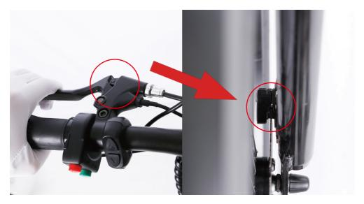
Loosen the bolt on the end of the disc brake caliper arm with the supplied allen wrench to adjust the brake cable tension. Once achieve the required tension mentioned above, fully secure the mounting bolt and the process is complete.
