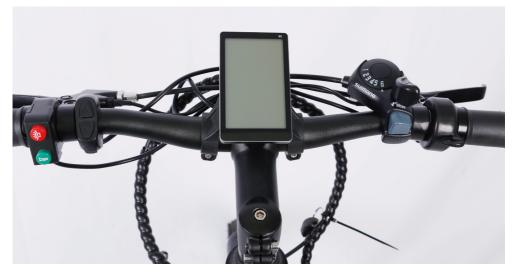
4.Tilt the LCD display to the optimal position and tighten the bolts.
