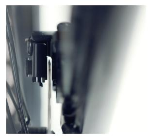
On the front disc brake caliper there are two bolts mounting it to the front fork. Loosen the mounting bolts until the caliper body is able to freely move side to side. Then squeeze the brake lever (this centers the caliper body over the rotor). While holding the lever, tighten the bolts. Release the brake lever, spin the wheel and check for pad rub. If there is no rubbing, the pads are aligned. Secure the mounting bolts to full torque and your work is complete.
