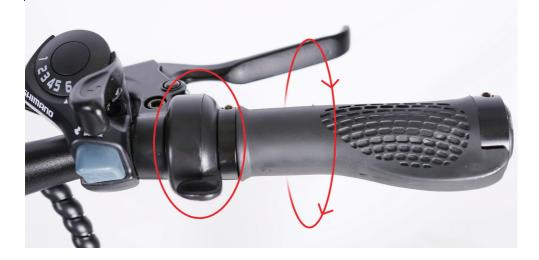
7.**Brake**—Brake the bike by squeezing the brake lever (**Notice:** as a safety feature applying either front or rear brake will disengage the motor.)
