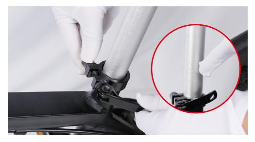
3.Close the quick release lever to secure the seat post and check that it cannot move. If needed, use the thumb nut to add tension to the clamp so there is some resistance when the lever is in line with the clamp bolt.
