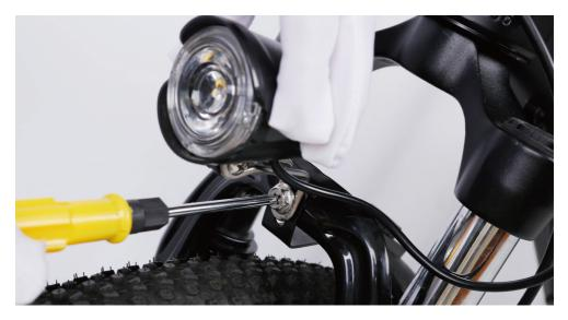
4.Center the headlight and adjust the angle slightly downwards to illuminate the road ahead and not blind oncoming traffic. Use the supplied Phillips-head screwdriver to loosen the headlight angle adjustment bolt, tilt the headlight to the optimal position, and then tighten in place securely.
