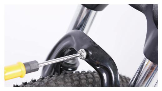
2.Place the fender in position. Pass the front fender mounting point under the front fork arch from the back of the front tire.
