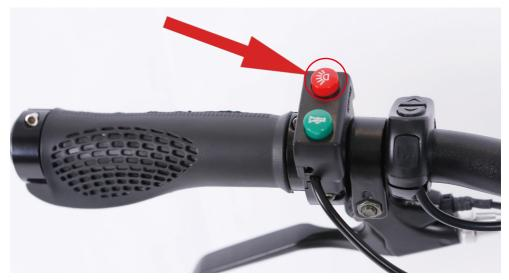
4.**Select the desired level of pedal assistance**—Select the level from 0-5 by pressing " ~ " and " ~ ". Level 1 corresponds to the lowest level of pedal assistance, and level 5 corresponds to the highest level of pedal assistance. Level 0 indicates pedal assistance is inactive. Start in PAS level 0 or 1 and adjust from there.
