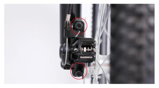
If the pads are still rubbing, we need to do some fine-tuning. Loosen one bolt at a time and adjust until there is a gap on either side of the rotor. Once the pads are not rubbing, fully secure each mounting bolt and the process is complete.
