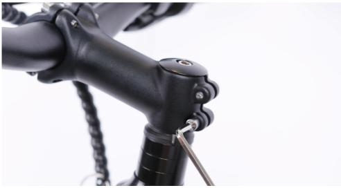
6.Tighten the bolt on the top of the steer stem with the supplied allen wrench.
