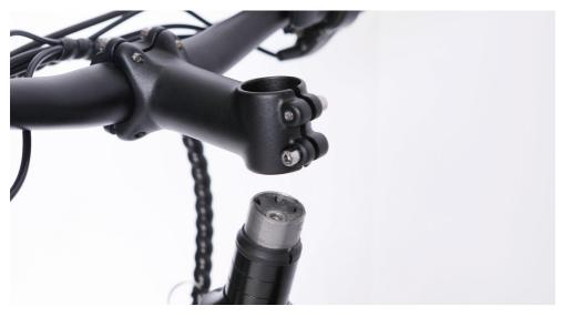
4.Pass the stem bolt through the washer mounting point and the stem mount, tighten with the supplied allen wrench part away.
