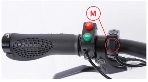
3.**Turn on the headlight** if needed or desired. Once the LCD Display is on, press the light button on the left side of the handlebar to turn the head-light on. Press it again to turn the headlight off.
