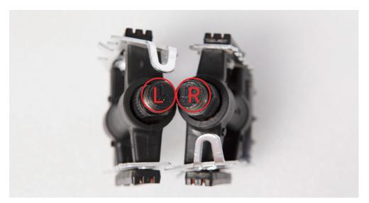
2. The right pedals threaded to tighten by turning clockwise. The left pedals reverse-threaded and tightens counterclockwise. Carefully thread the pedal onto the crank by hand slowly.
