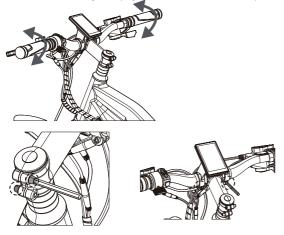
C.Adjust the handlebar height/angle to the desired position then use a 3mm hex key to tighten the screws securing it to the frame.
