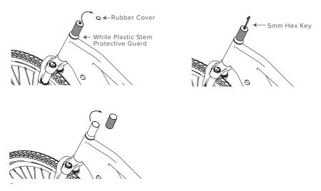
B.Place the handlebar stem onto the stem with the display facing upwards, replace the top cap and use a 5mm hex key to secure the handlebar stem. Reinsert the rubber cover back into the top cap.
