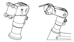
**Step 6:** Place the handlebar on the stem correctly. Center the handlebar and screw in the four stem faceplate bolts evenly, however do not tighten all the way down for further adjustment. (For Pace 500 )
