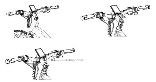
**Step 4.** Make sure the handle bars stay on the left side so after the handle bars are installed the cables come out of the frame to the left side of the bike. Make sure the cables are not twisted. (Reference below pic, For Pace 350 & Pace 500)
