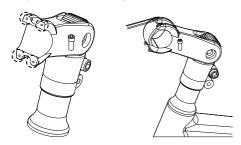
**Step 6:** Place the handlebar on the stem correctly. Center the handlebar and screw in the four stem faceplate bolts evenly, however do not tighten all the way down for further adjustment. ( For Pace 500 )
