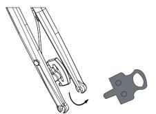
C.Carefully install the front wheel and make sure the brake rotor sits in between the braking pads in the brake caliper; the flat washer on the axle should sit outside the fork dropout.
