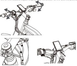
C.Adjust the handlebar height/angle to the desired position then use a 3mm hex key to tighten the screws securing it to the frame.
