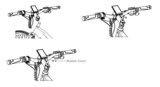
**Step 4.** Make sure the handle bars stay on the left side so after the handle bars are installed the cables come out of the frame to the left side of the bike. Make sure the cables are not twisted. (Reference below pic, For Pace 350 & Pace 500)
