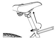
If needed, use the thumb nut to add tension to the clamp so there is some resistance when the lever is in line with the clamp bolt, but do not overtighten. Close the quick release lever to secure the seatpost and check that it cannot move. See the Adjusting the Seat section of this manual for more details.
