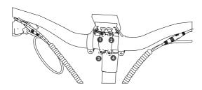
Step 10: Use 3mm hex key to tighten the display clamp to desired angle .
