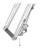
B.Remove the plastic insert card from the front brake caliper.
