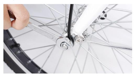
(4). Once you have tightened both axle nuts push the black plastic caps onto the front axle nuts.
