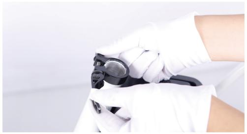
2.Insert seat post into seat tube. Adjust the seat post up or down to a comfortable height, while ensuring the seat post is inserted into the frame past the minimum insertion point.
