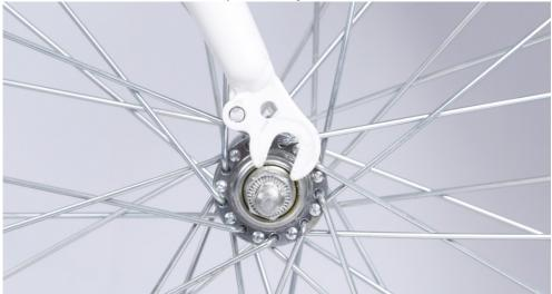
4.Line up the axle lock washers (These are the metal washer with a bent tab on one side) with the hole at each fork. **Notice:** These two special fork lock washers keep the wheel from falling off if the axle nuts ever loosen up! Tighten the axle nuts by hand.
