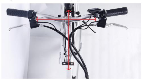
5. Tighten the bolt at the clamp with the supplied allen wrench.
