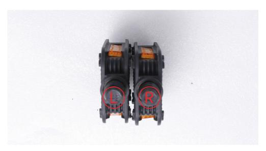
2.The right pedal is threaded to tighten by turning clockwise. The left pedal is reverse-threaded and tightens counterclockwise. Carefully thread the pedal onto the crank by hand slowly.
