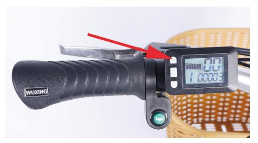
5.**Select the desired level of pedal assistance**—Select the level from 0-5 by pressing " $\nearrow$ " and " $\checkmark$ ". Level 1 corresponds to the lowest level of pedal assistance, and level 5 corresponds to the highest level of pedal assistance. Level 0 indicates pedal assistance is inactive. Start in PAS level 0 or 1 and adjust from there.
