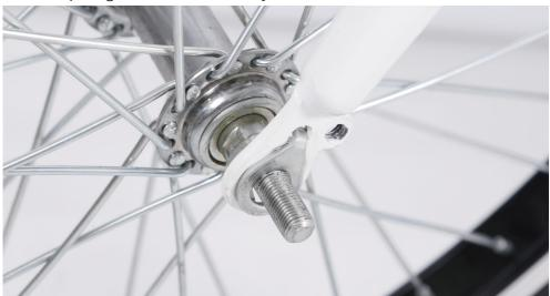
5.Once the lock washers are in place tighten both axle nuts with the supplied double open-end wrench. **Notice:** Before doing the final tightening of the axle nuts make sure the wheel is square and true with the forks.
