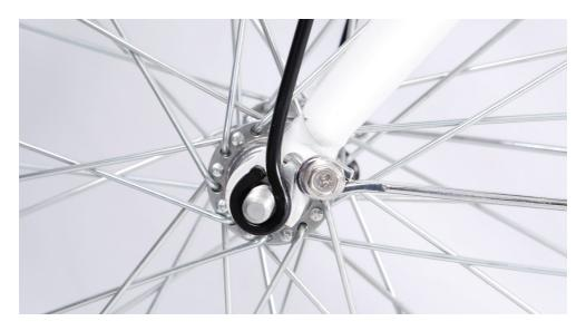
(3). Tighten both axle nuts with the supplied double open-end wrench.
