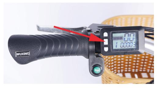
4.**Turn on the headlight** if needed or desired. Once the LCD Display is on, Press and hold "\(\sigma\)" button for approximately 3 seconds to turn on the headlight. Press and hold it for approximately 3 seconds again to turn the headlight off.
