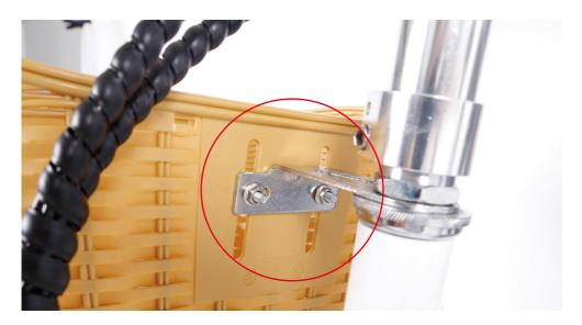
3. Fix the basket to the bottom bracket. Fit the bottom bracket into the curve of "bracket 4". Pass the bolt through "bracket 3" mounting point, the basket bottom mounting point and "bracket 4" mounting point. Tighten with the supplied screwdriver.
