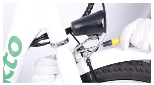
4.Attach the fender mounting arms to the front fork. Remove the mounting bolts from the fork. Pass the bolt through the arm mount and fork mounting point. Ensure the fender is centered and tighten both the mounting bolts.
