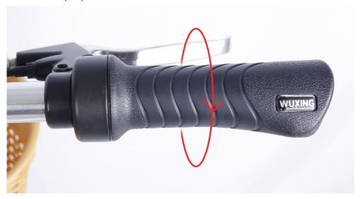
Do not use the throttle while dismounted. Avoid accidental application of the throttle while dismounted; anytime you are moving the bike while dismounted, ensure the bike is powered off to prevent accidental application of the throttle.
