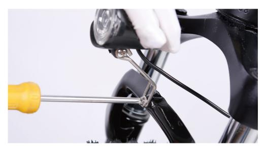
3.Center the headlight and adjust the angle slightly downwards to illuminate the road ahead and not blind oncoming traffic. Use the supplied Phillips-head screwdriver to loosen the headlight angle adjustment bolt, tilt the headlight to the optimal position, and then tighten in place securely.
