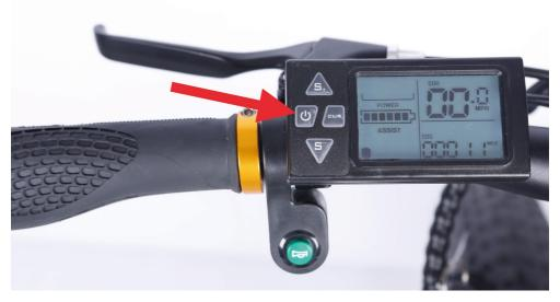
3. **Turn on the headlight** if needed or desired. Once the LCD Display is on, press "CUR" button to turn the headlight on. Press it again to turn the headlight off.
