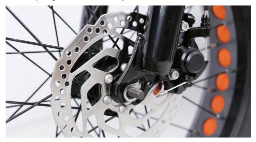
4.Tighten both axle nuts with the supplied double open-end wrench. **Notice:** Before doing the final tightening of the axle nuts, make sure the wheel is square and true with the forks.
