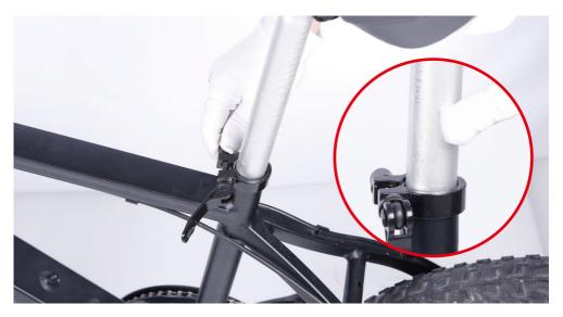
3.Close the quick release lever to secure the seat post and check that it cannot move. If needed, use the thumb nut to add tension to the clamp so there is some resistance when the lever is in line with the clamp bolt.
