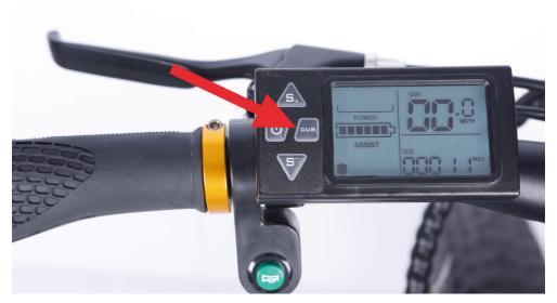
4.**Select the desired level of pedal assistance**—Select the level from 0-5 by pressing "S+" and "S-". Level 1 corresponds to the lowest level of pedal assistance, and level 3 corresponds to the highest level of pedal assistance. Level 0 indicates pedal assistance is inactive. Start in PAS level 0 or 1 and adjust from there.
