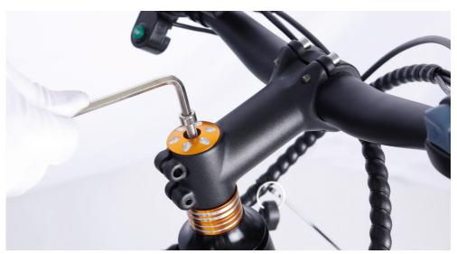
5.Align the stem so the handlebar is perpendicular to the front wheel. Use the allen wrench to tighten the stem clamp bolts evenly (a half turn at a time alternating between the two bolts).
