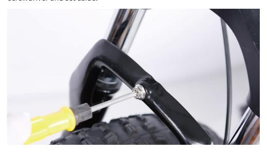
2.Attach the headlight to the fork arch. Pass the headlight mounting bolt through the headlight mount and the fork arch mounting point. Thread the locknut onto the bolt and tighten with the supplied screwdriver.
