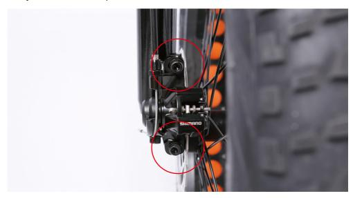
If the pads are still rubbing, we need to do some fine-tuning. Loosen one bolt at a time and adjust until there is a gap on either side of the rotor. Once the pads are not rubbing, fully secure each mounting bolt and the process is complete.
