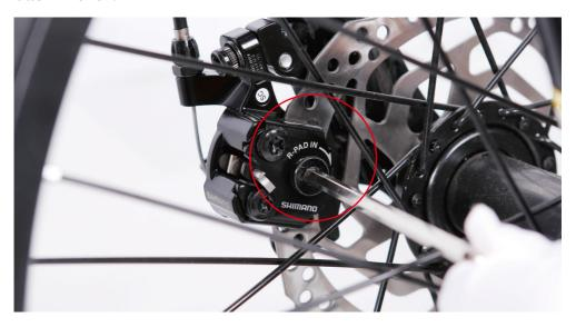
2.Check and adjust the travel at the brake lever at the handlebars. Typically, the pads should feel like they are contacting the rotor at a minimum of 1/2 the lever travel. We will get it by adjusting the brake cable tension.
