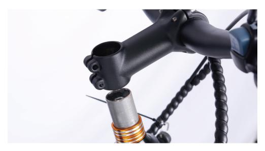
4. Pass the bolt through the washer mounting point and the stem mount, tighten with the supplied allen wrench part away.
