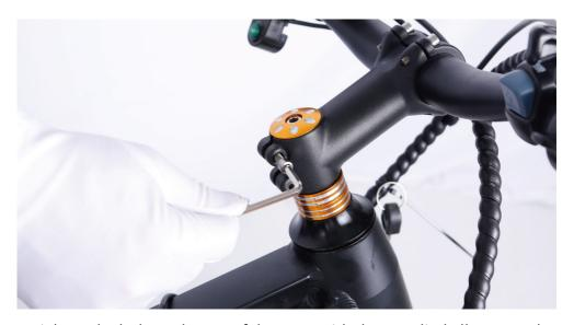
6. Tighten the bolt on the top of the stem with the supplied allen wrench.
