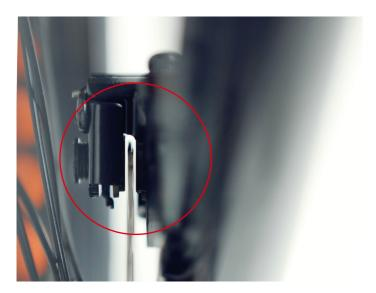
On the front disc brake caliper there are two bolts mounting it to the front fork. Loosen the mounting bolts until the caliper body is able to freely move side to side. Then squeeze the brake lever (this centers the caliper body over the rotor). While holding the lever, tighten the bolts. Release the brake lever, spin the wheel and check for pad rub. If there is no rubbing, the pads are aligned. Secure the mounting bolts to full torque and your work is complete.
