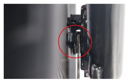
3.Line up the axle lock washers (These are the metal washer with a bent tab on one side) with the hole at each fork. **Notice:** These two special fork lock washers keep the wheel from falling off if the axle nuts ever loosen up! Tighten the axle nuts by hand.
