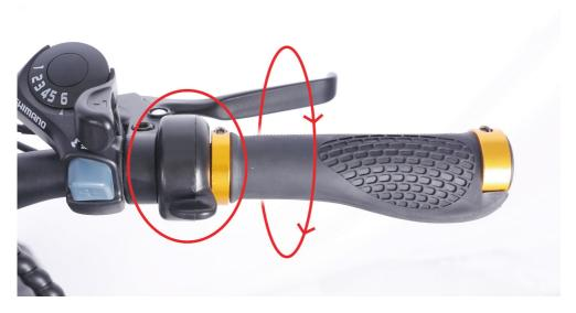
7.**Brake**—Brake the bike by squeezing the brake lever (Note: as a safety feature applying either front or rear brake will disengage the motor.) 8.**Cruise Control**:
