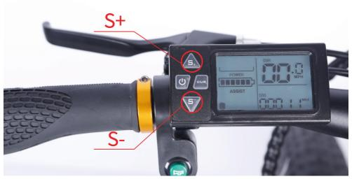
5.**Begin riding carefully**—Hold handlebars and start pedaling on a flat surface, in a low gear (1 or 2), most riders should be able to begin pedaling the bike with pedal assist level 0 or 1. You may also use the throttle to accelerate and maintain your desired speed.
