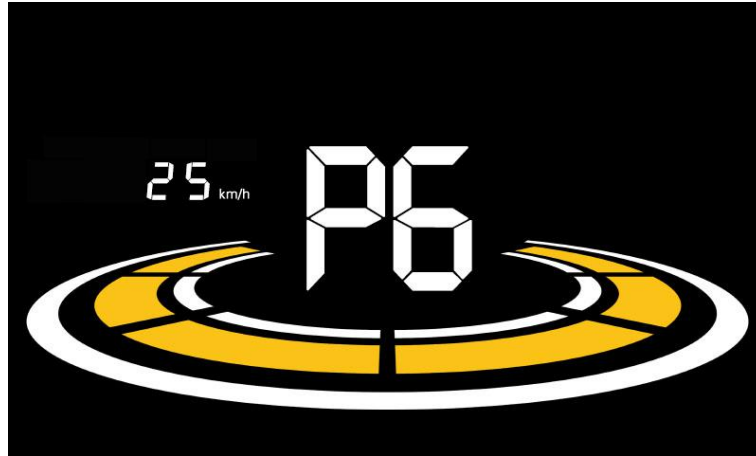
Figure 6-5 Speed limit setting interface
