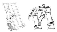
B. Align front fender to the screw holes.
