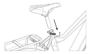
If needed, turn the adjustment nut clockwise to increase tension to the clamp to ensure proper clamp force when the lever is in line with the clamp bolt, but do not overtighten. Close the quick release lever to secure the seatpost and check that it is secure. See the Adjusting the Seat section of this manual for more details.
