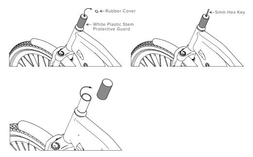
**Step 3.** Place the handlebar stem onto the stem with the display facing upwards, replace the top cap and use a 5mm hex key to secure the handlebar stem. Reinsert the rubber cover back into the top cap.
