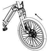
E. Use the 6mm hex key to tighten the barrel shaft bolt with strength of 8-10N  $\,$
