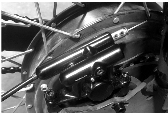
NEW CALIPER INSTALLED WITHOUT DUST COVER
