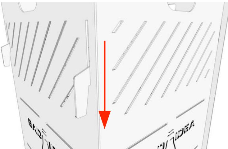
Slide the tabbed panel down into the slot locking the two panels securely together.
