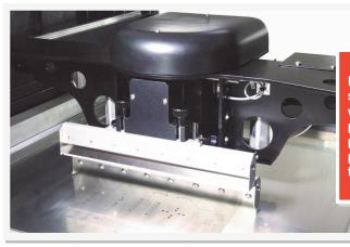
Independent, dual squeegee print head with programmable printing speeds and pressure for quality printing results each time
