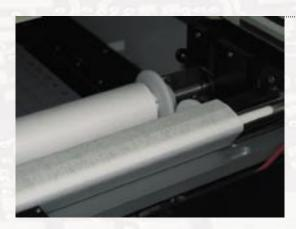
Stencil cleaning is applied wet, dry and with vacuum, in order to keep the smallest of apertures free from paste residues during the print process.
