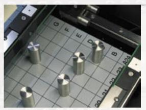
The magnetic support pins provide a simple and costefficient solution for flat substrates. The pins are also available as vacuum suction heads or as centre pins.
