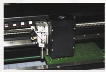
The PCB stop can be freely positioned. The appropriate position is automatically calculated from the dimensions and form of the PCB.
