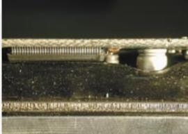
The modular "Vacunest" system is the optimum support device for double-sided populated board assemblies. It adapts automatically to any board surface structure and therefore consistently distributes the pressure over the entire area.
