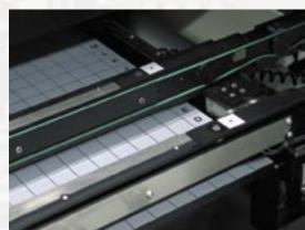
The thickness of the PCB or the substrate does not interfere with the function of the clamping system. The design of the clamping system ensures full stencil contact with the PCB.
