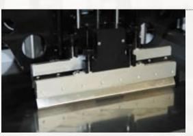
The print head uses two independently controlled floating head squeegees. Printing speeds and pressures can be individually programmed for each forward and reverse printing directions. Squeegees made from metal and rubber or flood blades can be used for widths of up to 608 mm. Squeegees with different angles (60° or 45°) can be delivered.
