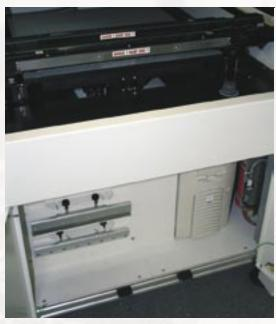
Designed for easy accessibility from the front: replenishment of cleaning liquid, exchange of paper rolls or other regular maintenance work (right).
