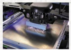
The basic printing machine can handle a variety of features: rubber, metal or flood blade squeegees, stencil frames with small dimensions to larger ones of 29 x 29", as well as substrates from 0.3 to 5 mm in thickness and outer dimensions of 608 x 540 mm. Also, customer-specific solutions can be provided within a very short time scale.
