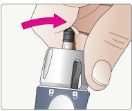
Loosen the internal part of the Nozzle by pushing it firmly to one side.
