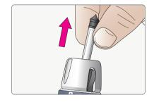
Remove the internal part of the Nozzle and discard it together with the nozzle.
