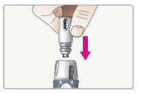
Firmly push the Nozzle into the Nozzle I ock.
