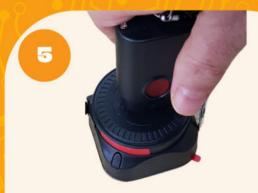
To deactive the alarm place the magnetic lock detacher on the unit, Push the red button and a beep will sound. The alarm is now off.
