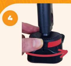
With the magnetic detacher still in place, twise the base counter clockwise.
