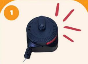
The unit will let off a short chirp of the alarm to indicate a low battery.
