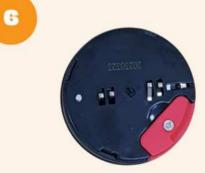
Remove the red battery cover and replace the battery CR-2032
