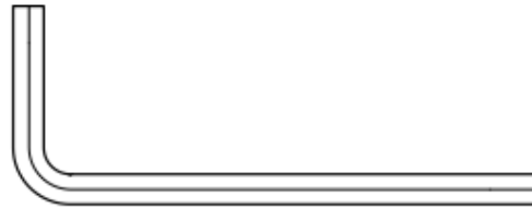
Camera Mounting Tool - 3/16" Hex Key F545
