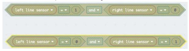
☐ The right and left line sensor variables are loaded with sensor data at the start of each repetition of the loop.
