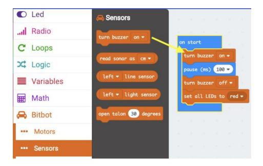
☐ Continue to drag the blocks into the **on start** section. Once your code is loaded onto the micro:bit in your Bit:bot robot and the power is switched **ON**, these commands will be run.
