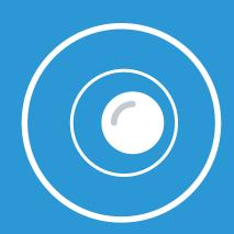
Make sure your mount and tripod are level. Your setup will be level when the bubble is in the middle circle.
