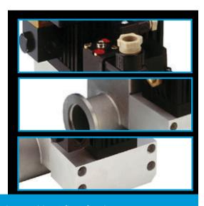
Soft-start, pneumatically operated, in-line valves with interchangeable orifices for the controlled pump-down of processes where turbulent flow can cause problems with particulate contamination. Slave and master valve combination allows slow initial pumping to minimise disturbance. Both slave and master valves require separate pneumatic connections.
