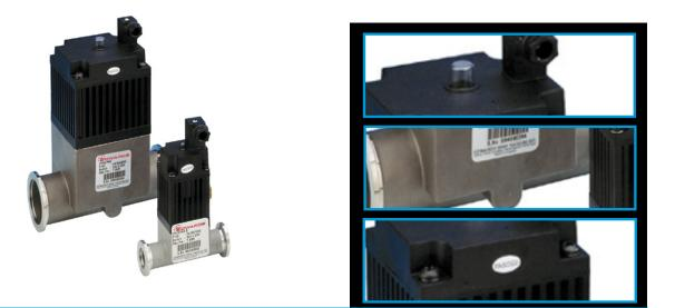
The Edwards range of in-line single acting cylinder, spring return pipeline valves are designed for high speed actuation from standard pneumatic lines, and are offered in sizes NW16, 25, 40 and 50. They are available with aluminium or stainless steel bodies with either O-ring (shaft seal, aluminium only) or bellows sealed.
