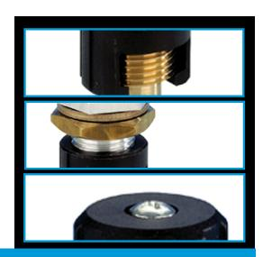
The AV5A is manufactured in aluminium alloy. It has a control knob attached to a screw-actuated plunger: turn the control knob clockwise to close the valve. A nitrile 'O' ring seals the plunger to the valve body.
