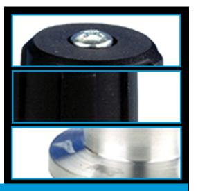
The AV10K is manufactured in aluminium alloy. It has a control knob attached to a screw-actuated plunger: turn the control knob clockwise to close the valve. A nitrile 'O' ring seals the plunger to the valve body.
