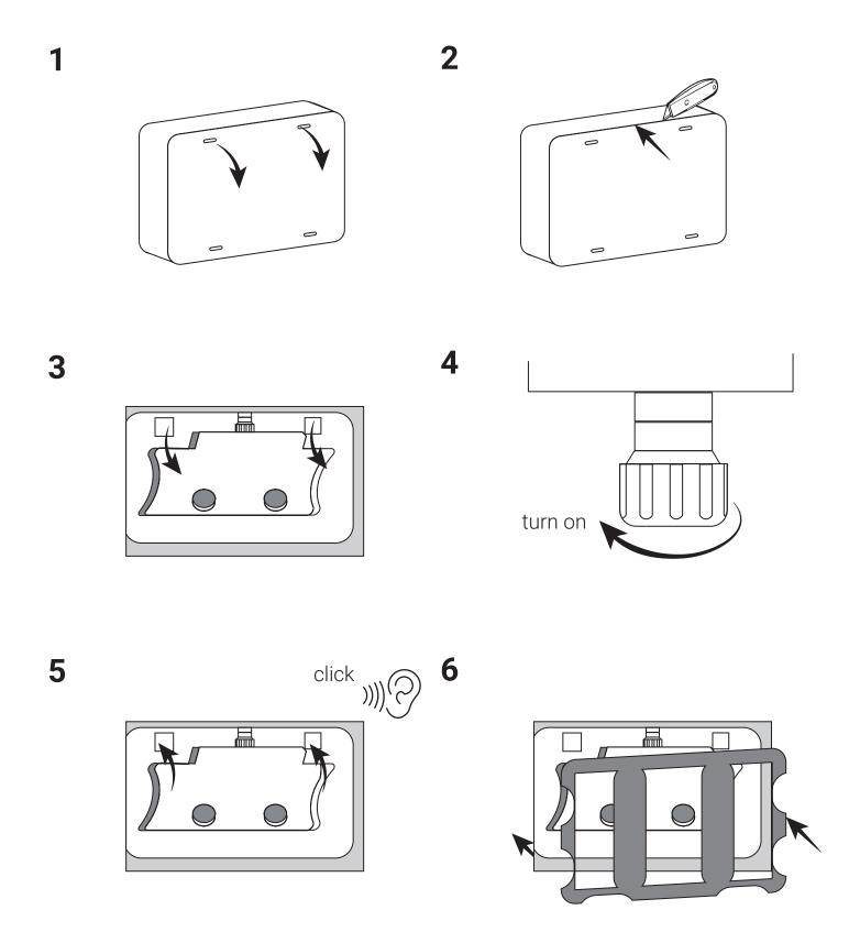
NOTE: This flushplate must be used with the back plate provided as a whole set.
