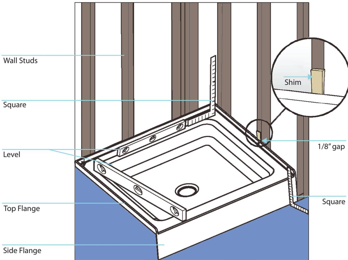
5. Place drop cloth in bathtub and stand inside the shower base to press it to the floor when securing to the wall studs.
