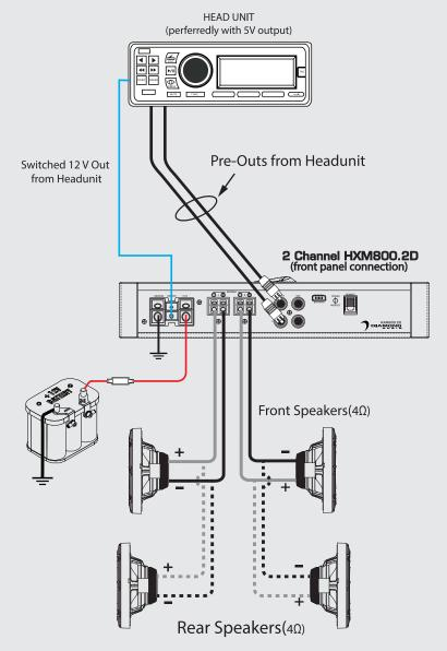
Total speaker impedance Total Speaker Impedance (MIN  $2\Omega$ )
