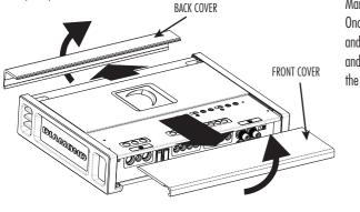
Mark Amplifier Mounting Holes: Once the covers are removed, use a pencil and mark the mounting locations. Both front and rear. Once marked, drill 1/8" holes for the included mounting screws. (see below)
