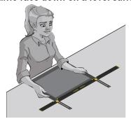
B. Move the right arm of HIP to be flush with the end of the crossbar. Tighten to secure in place. A ledge is formed on the end that will be used in step 3.
