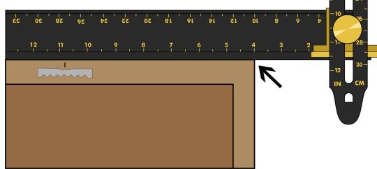
D. Move the left arm of HIP to the frame center. Slide arm up until hook catches the center of the frame's hanging mount or wire. Tighten knob to secure arm in place.
