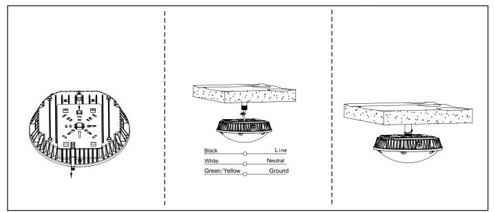
Surface-mounted with side-wiring
