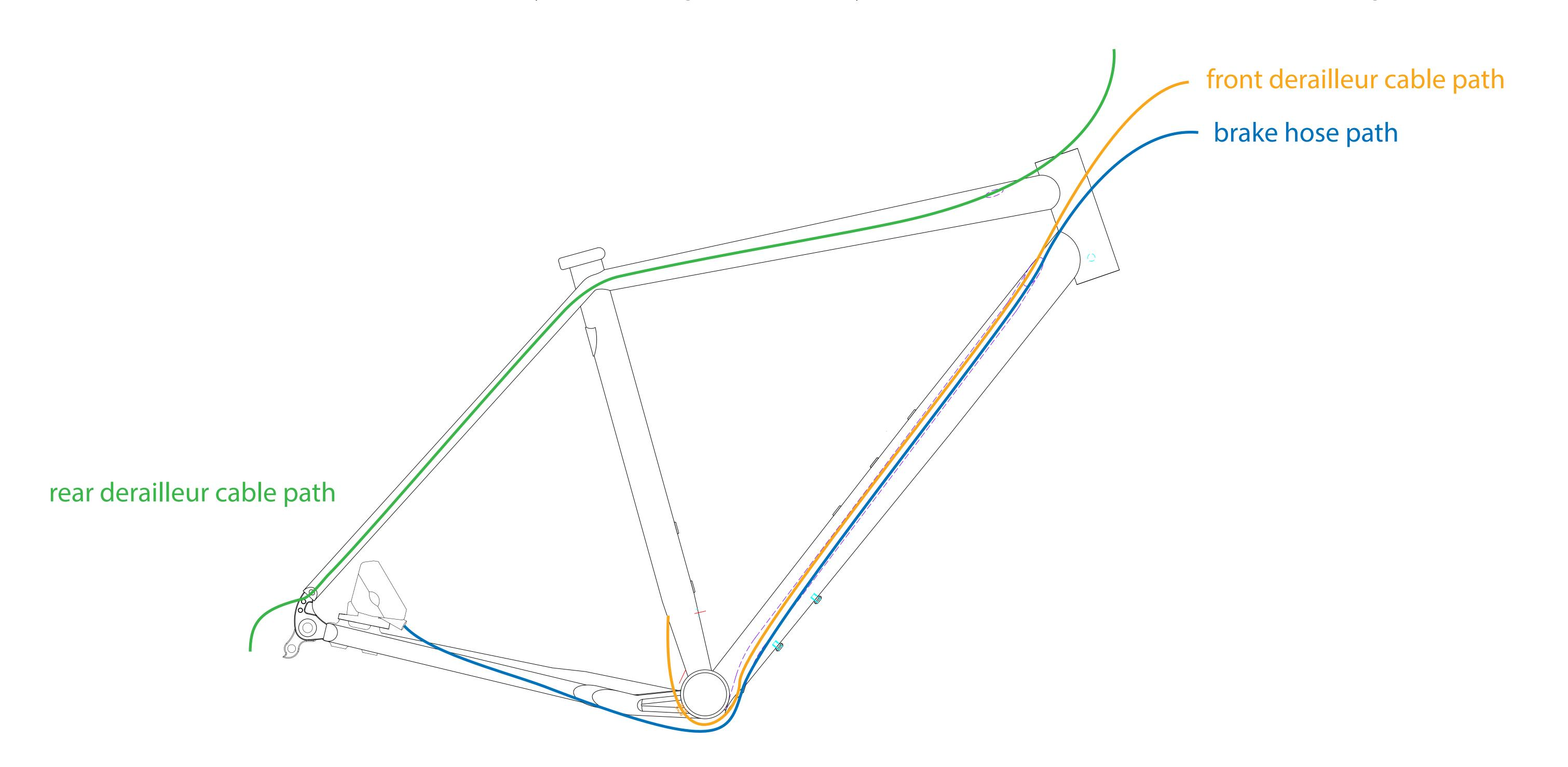
We've prerouted a gear cable through the top tube and seatstay of your frame. Should this not be in place, we encourage you to start by routing this cable from the top tube cable port, through the seastay, and exiting at the dropout. A slight amount of bend in the cable will allow you to rotate and guide the cable along the drive side seatstay.
