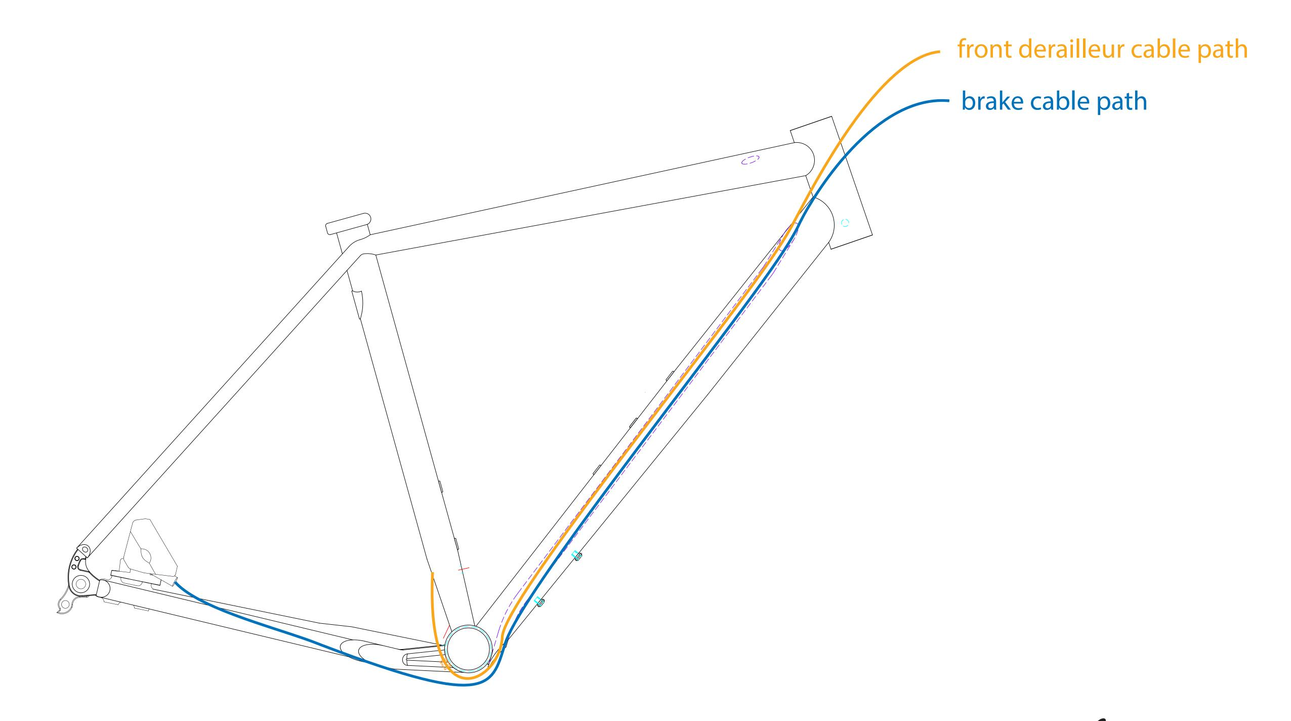
Should you have ordered your mechanical spec frame with the internally routed dropper option, there will be a small cable port on the back of the seat tube, just above the bottom bracket shell.
