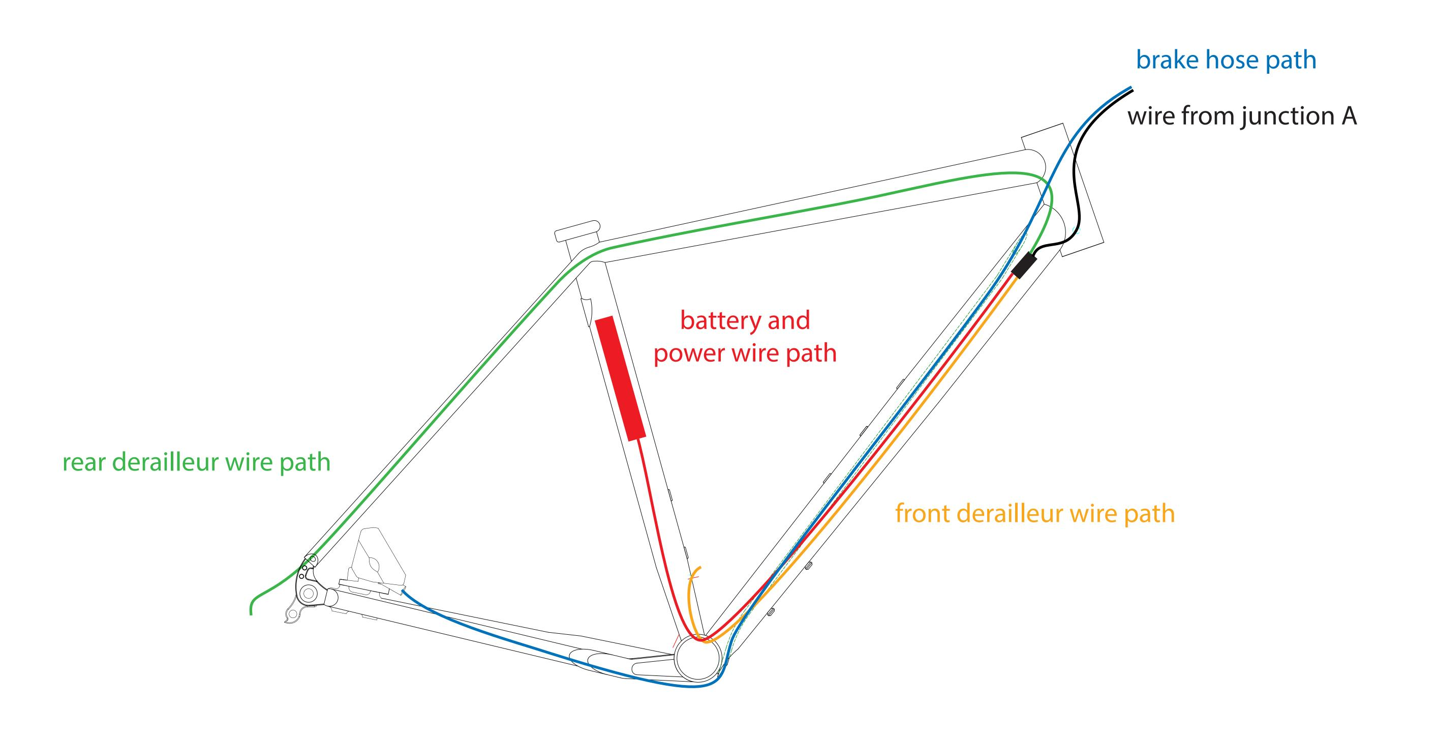
We've prerouted the 1600mm Di2 wire through the top tube and seatstay of your frame. Should this not be in place, we encourage you to use a Park Tool routing cable or similar device to aid the transfer of the Di2 wire from dropout to the headtube. It may be helpful to position the frame upside down as the cable connector passes through the seat-stay / top tube junction. Gravity is your friend and helps minimize snagging of the plug.
