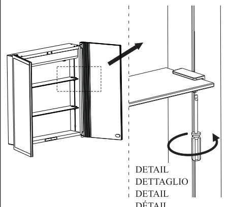
LOOSEN SCREW TO ADJUST SHELF TO DESIRED LOCATION AND TIGHTEN IT.
