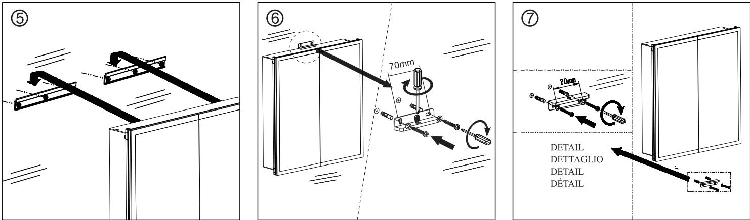
5. Lift cabinet onto mounting plate.
