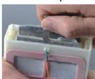
9. Insert new electrode plate correctly (note: the longer end is near the water inlet)
