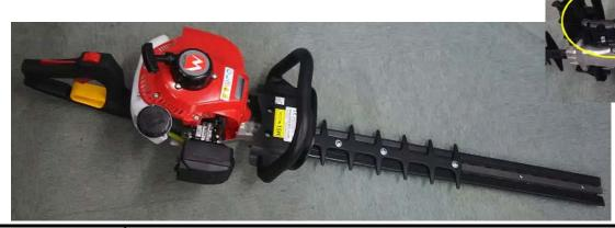
Front exhaust muffler extension (less harm for operator &
