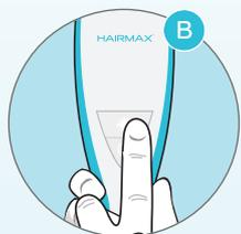
• **Turn on the LaserComb** by pressing the power button and hold until power button light turns on. Next, press the laser button until it lights up. That means the LaserComb is ready for use (Figure B).
