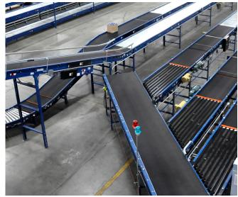
End pulleys are 2-1/2" diameter to **reduce gaps** between units for small product transportation. A belt-low configuration eliminates the guard rail on floor-mounted conveyors and reduces guard rail requirements for overhead units.
