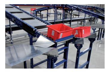
No conveyor is more economical or maintenance free than TGW Systems Controlled Flow Gravity roller conveyor. With gravitational pull causing product movement, and pneumatic components providing control, this is the most efficient and reliable decline accumulation conveyor available. It eliminates expensive decline belt conveyors while still providing controlled accumulation. Gravity conveyor is easy to install and without motors is much less expensive and much quieter than powered equipment.
