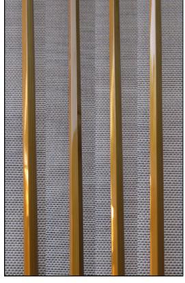
Various views of a butt section finished with Gorilla Glue. Taken at an angle to show reflections.
