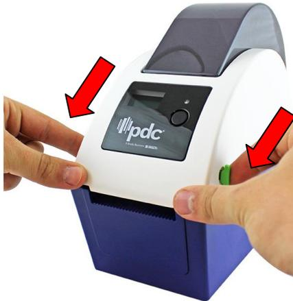
3. Separate the media holders to the wristband roll width.
