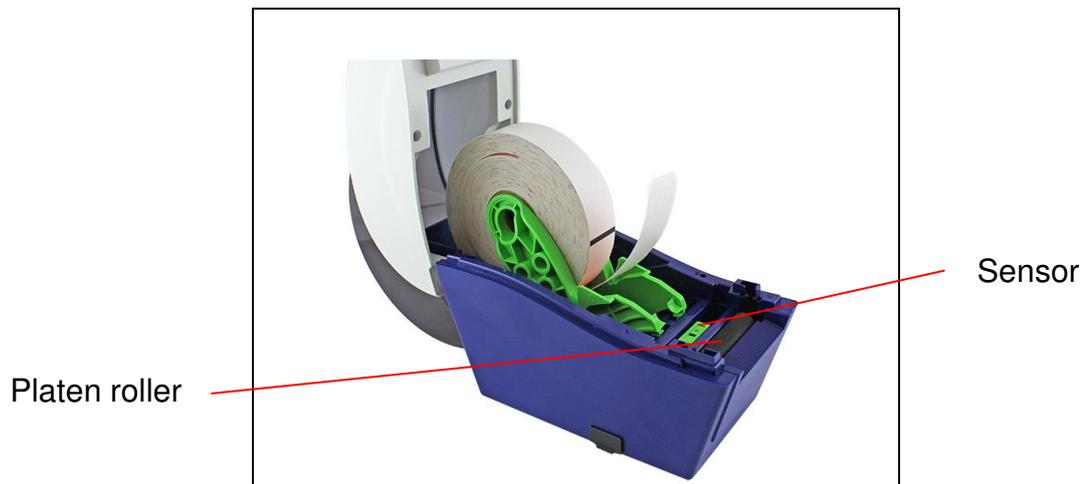
5. Place the paper, printing side face up, through the media guides, media sensor and place the wristband leading edge onto the platen roller.
