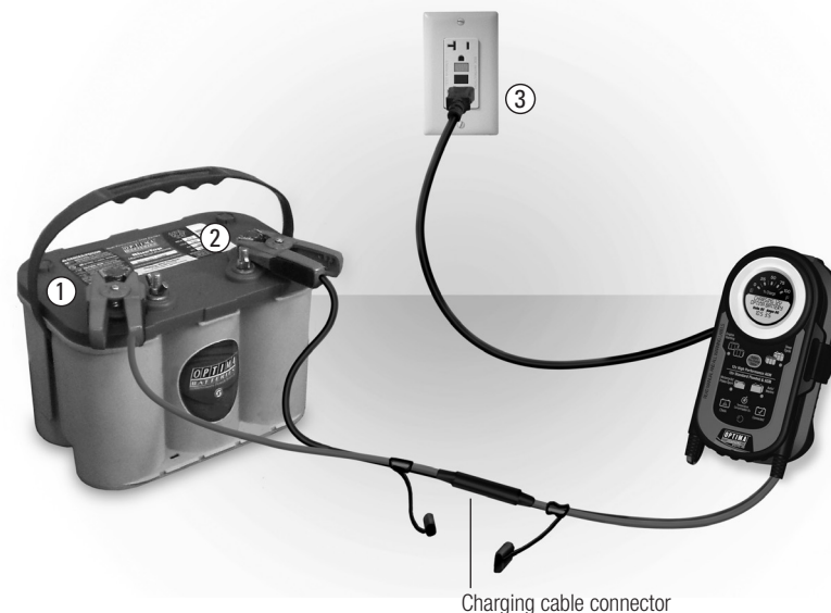
Pictured: Typical DC charging clamp connections for a precharge status, charging or just maintaining a fully charged battery with the DC charging clamps out of vehicle.
