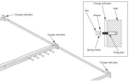
Put the canopy frame into position, ensure that feet are flat on the floor and the tracks are level using a sprit level. Mark the wall with the position of the 4 holes of each wall plate.
