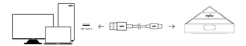
\*Pyramid will flash a red LED light when connecting. When connected to the mouse, the pyramid will have a solid white LED light.
