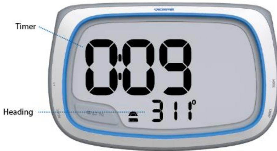
In timer mode the device displays the timer on top and heading at the bottom. In the above display there is only 9 seconds left before the start and heading is 311°.
