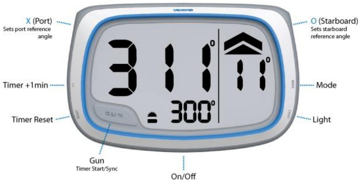
There are eight buttons on the device O(Starboard), X(Port), +1, RESET, MODE, LIGHT, GUN and PWR.
