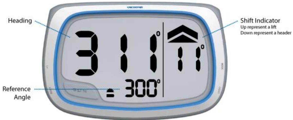
In compass mode the device displays heading on top, reference angle at the bottom and the shift indicator on the side. In the above display the heading is  $311^\circ$ , the starboard reference angle is  $300^\circ$  and the shift indicator shows a lift of  $11^\circ$ .
