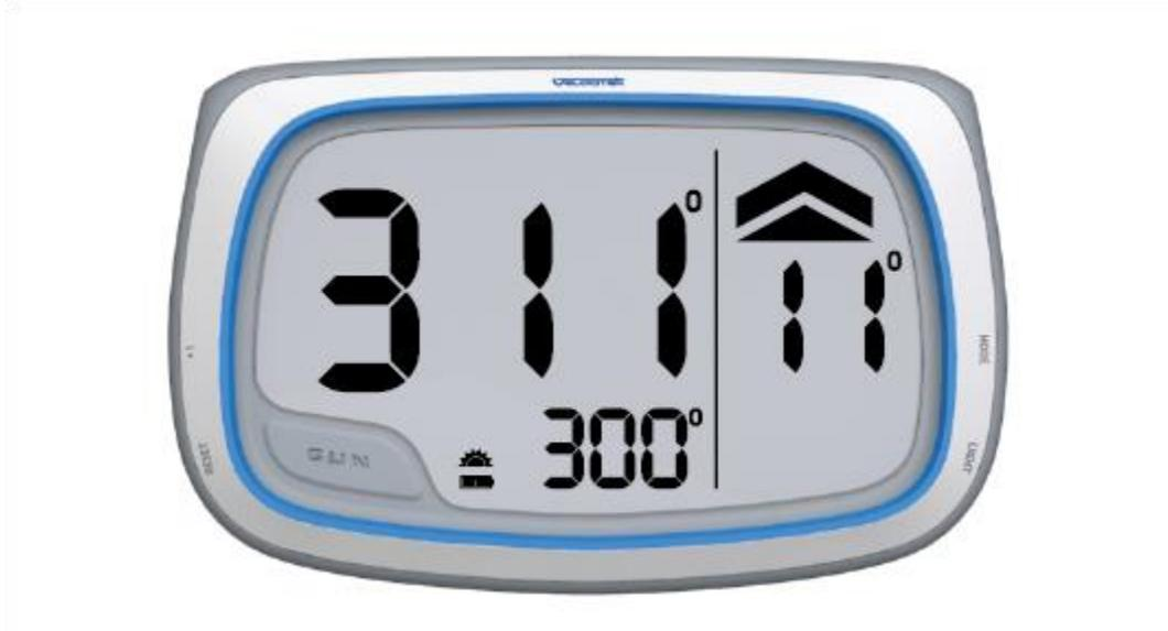
The Velocitek Shift is an electronically gimballed compass that helps sailors identify wind shifts. The Shift stores starboard and port tack reference angles and displays the difference between the current heading and the reference angle to help monitor wind shifts. The Shift's sensor suite consists of a magnetometer that is electronically gimballed by a gyroscope and an accelerometer. As a result the compass response is much faster and smoother than the traditional sailing compass.
