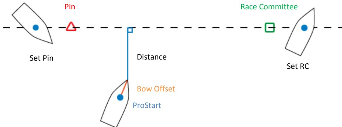
The above illustration provides a graphical definition of distance to start line and how you can set it.
