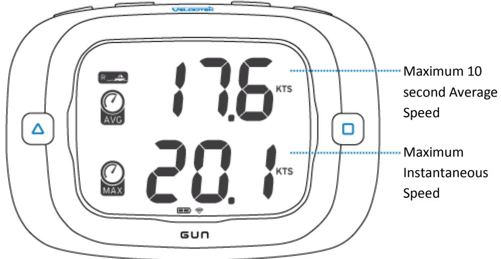
Display both your instantaneous and 10 second average maximum speed by holding **MAX**. To reset the maximum speeds, press **RESET** while holding **MAX**.
