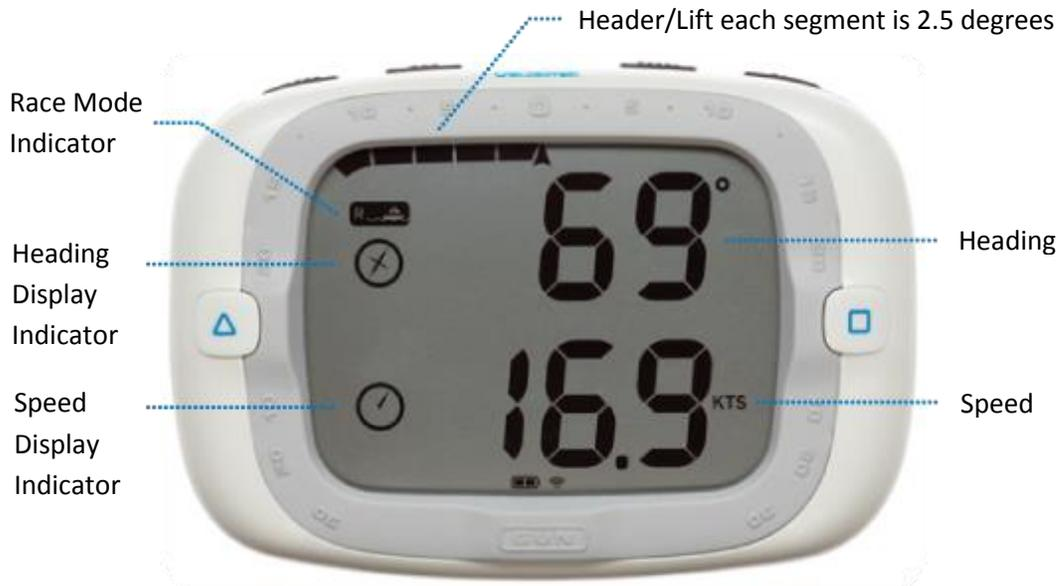
The race mode displays information crucial during the race, speed, heading and header/lift to the sailor.
