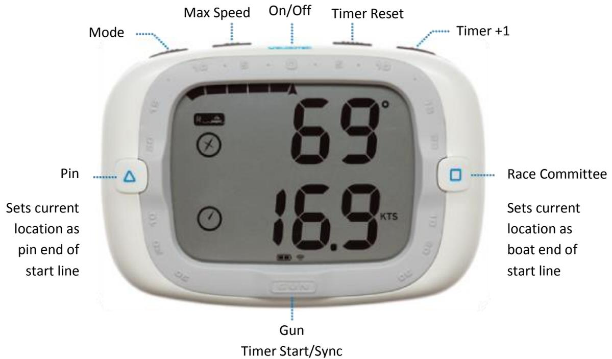
There are a total of 8 buttons on the ProStart as illustrated above. The buttons will be referred to in capitalized blue text throughout this document as follows, **PWR**, **MODE**, **MAX**, **RESET**, **+1**, **PIN**, **RC** and **GUN**.
