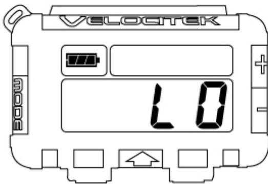
Time to replace the batteries
