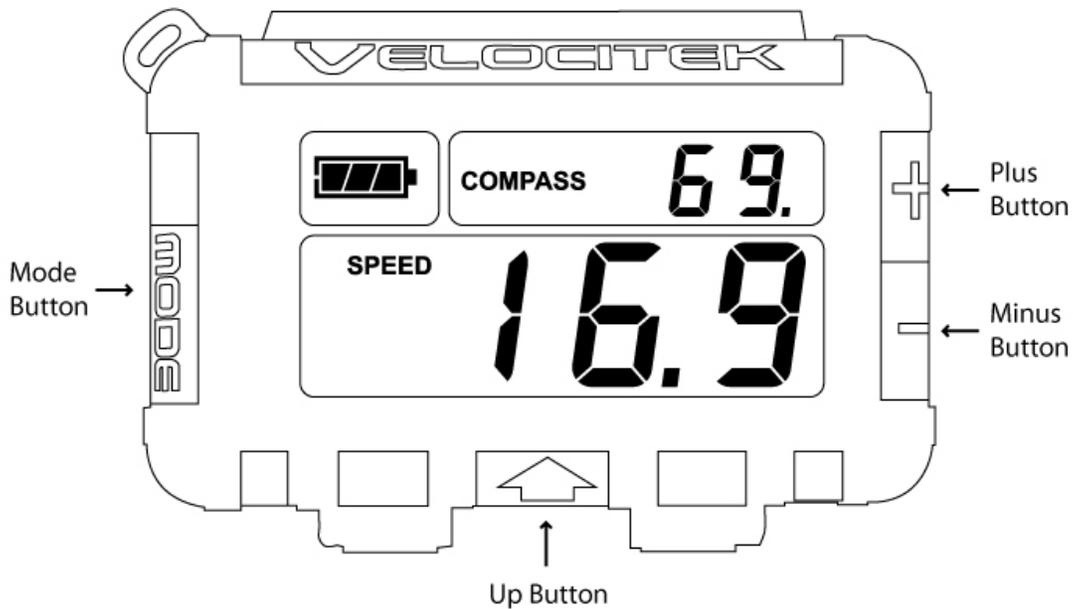
The SC-1 is controlled by four different capacitive touch sensors. These touch sensors detect the presence of your thumbs when they are placed on top of the regions shown in the diagram. The captions on the above diagram indicate how the different touch sensors will be referred to in the rest of this manual.
